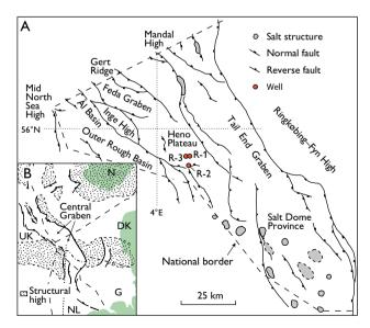
Fig. 1. **A**: Present structural framework of the Danish sector of the Central Graben. **R-1**, **R-2**, **R-3**: Ravn-1, -2 and -3 wells. **B**: Overview of the North Sea area. Green: Land. Modified from Johannessen (2010).
