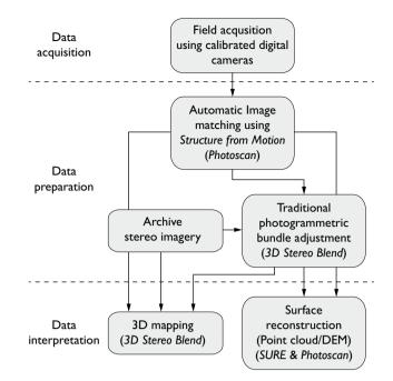
Fig. 3. Schematic flow diagram summarising the typical 3D-mapping workflow from data acquisition to photogrammetric data preparation and interpretation.
