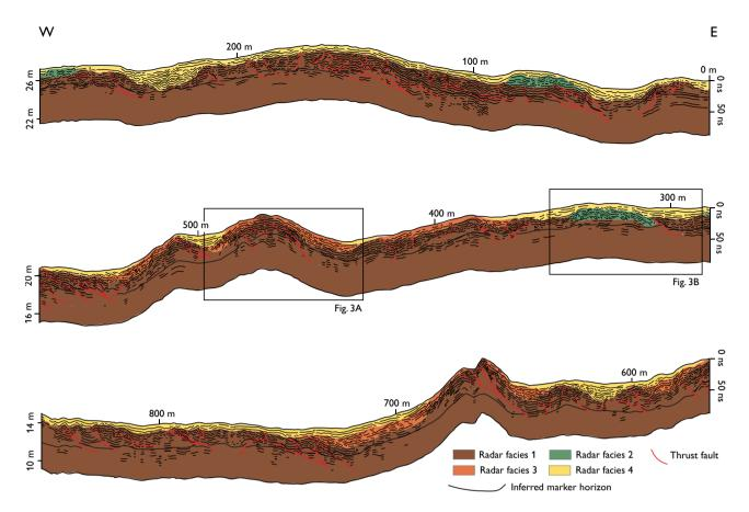
Fig. 2. Interpretation of the ground-penetrating radar profile LINE05. The scale to the left shows metres above sealevel. The scale to the right shows twoway travel time in nanoseconds. The black line is an inferred marker horizon used for structural analysis. The vertical exaggeration is 1:4. The black boxes indicate details shown in Fig. 3.
