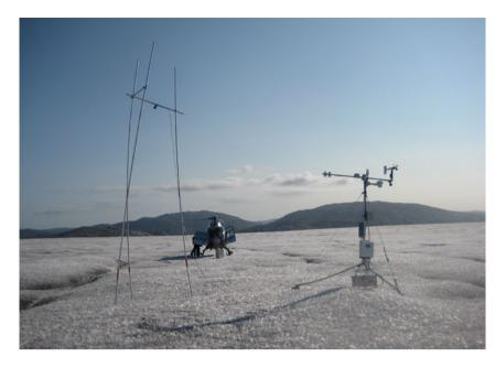
Fig. 2. South Greenland PROMICE automatic weather station at the end of the 2013 melt season. From the stakes to the left of the weather station, the amount of melt (*c*. 4 m) is directly visible. The melt is also measured with a pressure transducer system drilled into the ice.
