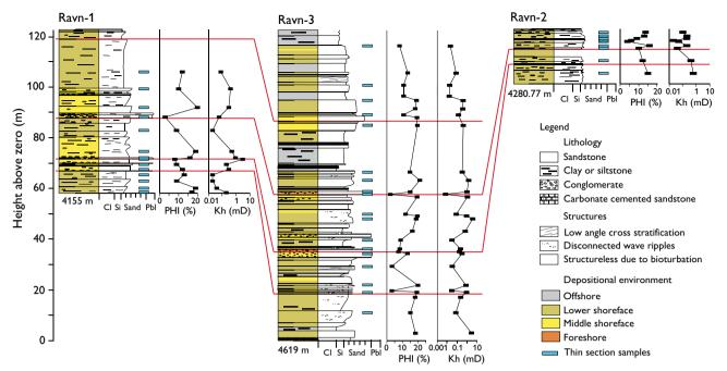
Fig. 2. Correlation panel of the cored parts of the Ravn-1, -2, and -3 wells. The Ravn-1 and Ravn-2 logs are modified from Johannessen (2010), whereas the Ravn-3 core was logged for this study. The depositional environment described in the Ravn-3 well (Panterra 2011) is based on ichnofacies. **PHI**: Heporosity. **Kh**: horizontal permeability. **Cl**: clay. **Si**: silt. **Pbl**: pebble.
