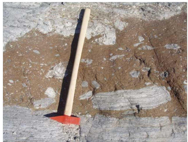
Newly discovered solid sphalerite ore in brecciated host rock near Maarmorilik (GEUS)
