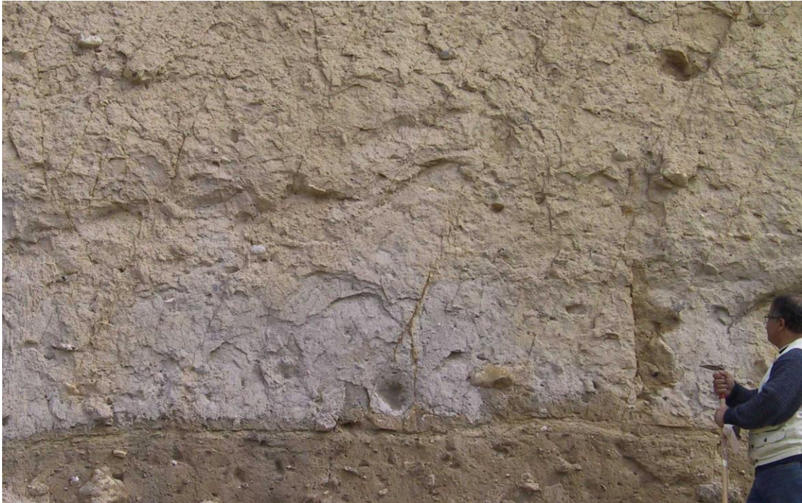
Figure 22. Clayey till profile from a gravel pit, Sjælland. Sets of sub-vertical fractures can clearly be recognized (Photo: K.E.S. Klint).
