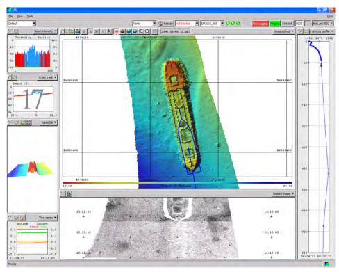
data. There are graphical windows for quality checking of sensor input and the data produced. Sound speed at sonar head and sound speed profile input are interfaced and handled correctly in real time.
