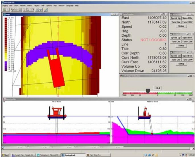
**DREDGEPACK®** runs on cutter suction, hopper, excavator and bucket-style dredges. It can store a history of the dredge's position, draft, digging tool depth and digging status in order to meet reporting requirements. **DREDGEPACK®** has been designed to run with a minimum of user intervention. Make sure you are maximizing your dredge's efficiency with **DREDGEPACK®**
