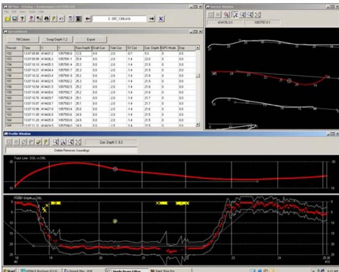
**EDITING:** The SINGLE BEAM EDITOR program is used to quickly review your survey data and to automatically and/or manually remove outliers. Sounding data is simultaneously displayed in plan, spreadsheet, and profile views with the channel design info drawn in the backgrounds. Routines developed by HYPACK® in collaboration with the U.S. Army Corps of Engineers to integrate water level corrections based on RTK GPS elevation info are a standard part of package.
