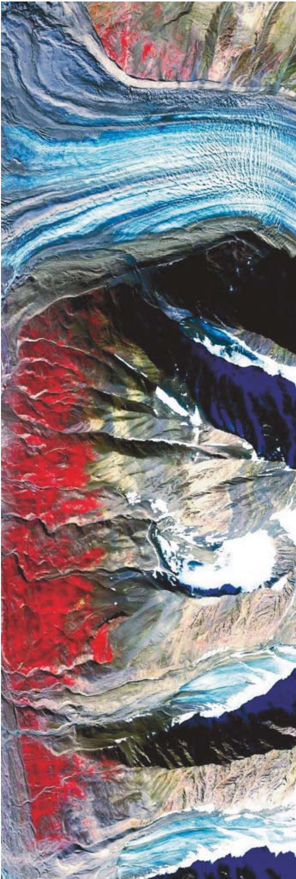
False colour 'quicklook' of HyMap TM data west of Mestersvig, July 2000. Grey and brown colours are sediments, bright red colours are vegetation and ice-blue colours are glaciers. Size of field: 10 x 2.3 km.
