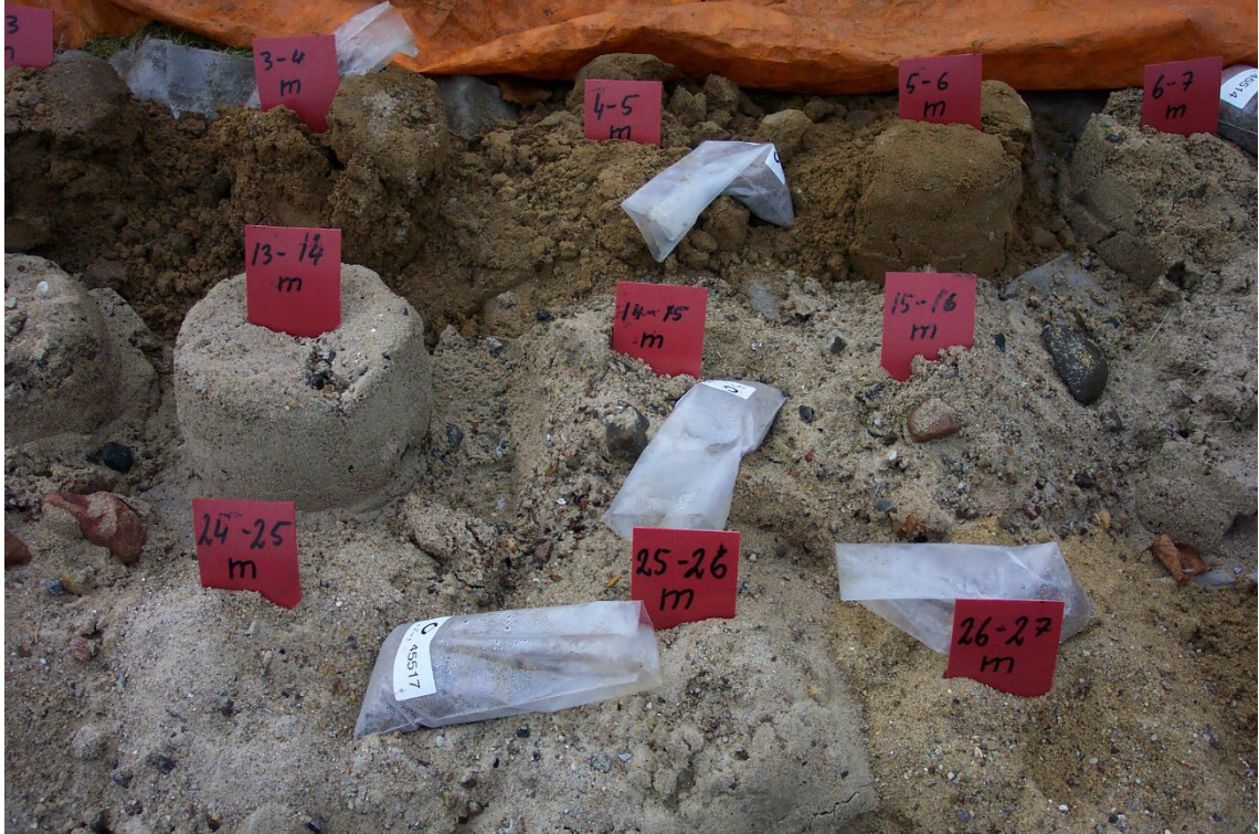
Figure 4. Sediment samples from the drilling process laid out so the lithological sequence can be easily followed, ensuring accurate geological description on-site.
