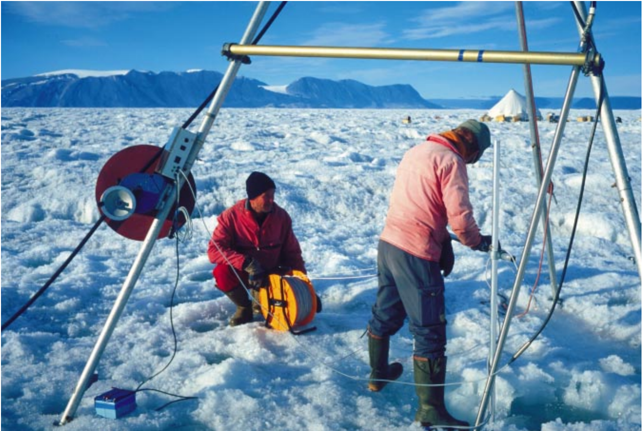
Fig. 5. Logging of ice thickness in drill hole at stake 0296 on Nioghalvfjærdsfjorden glacier.
