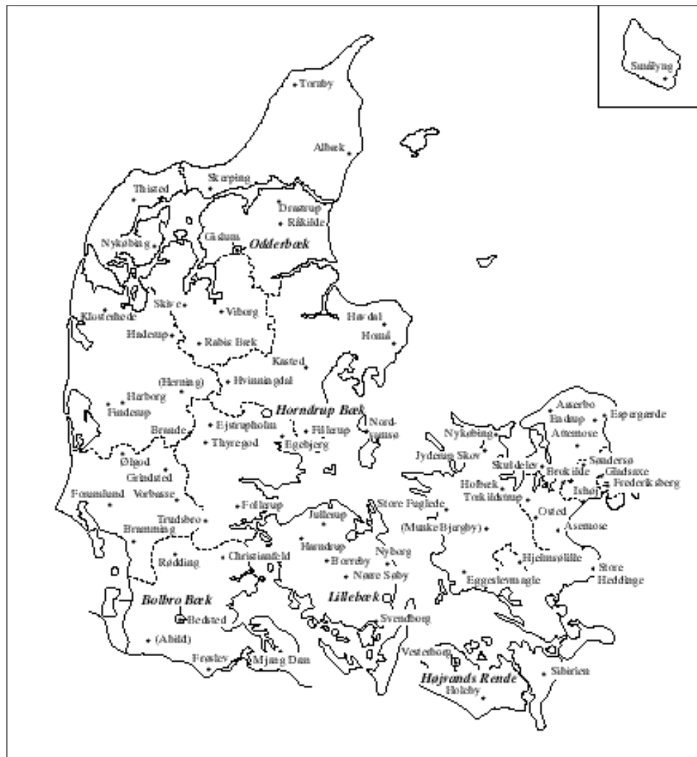
Figure 6.1 Groundwater monitoring sites (GRUMO) (·) and agricultural monitoring catchments (LOOP), level 3 + 4 (○) in Denmark 1998–2003. The groundwater monitoring sites Munke Bjergby, Abild and Herning have been placed on hold since the end of 1996 (shown in parentheses) except that a very limited programme is being continued in a small number of screens in the 3 sites. These sites are being replaced by 3 new groundwater monitoring sites, Jyderup Skov, Frøslev and Klosterhede.
