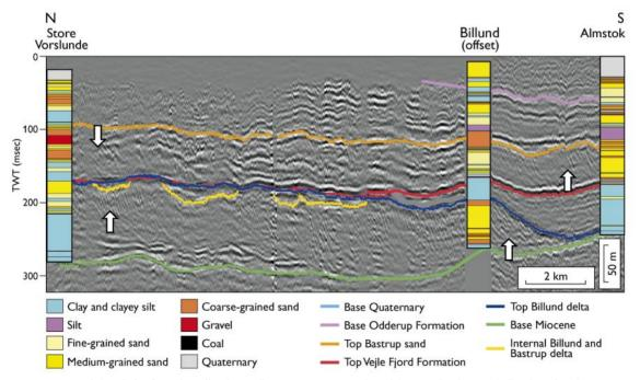
Fig. 3. Seismic section with boreholes from the Billund area illustrating two prograding deltaic sand-rich units (Billund sand and Bastrup sand). The grain size of the penetrated succession is indicated by different colours. Note that the parallel clinoformal seismic reflection pattern (arrows) always correlates with sand. Seismic data courtesy of COWI A/S and Rambøll A/S.
