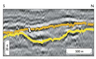
Fig. 5. Seismic section showing shingled, seismic reflection pattern (arrow) within a channel structure. Similar structures have been found on 3D seismic data from Canada (Posamentier 2005) and represent lateral accretion of a point bar. Seismic data courtesy of COWI A/S.
