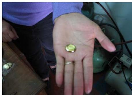
The final result: A pure gold pellet produced without use of mercury.
