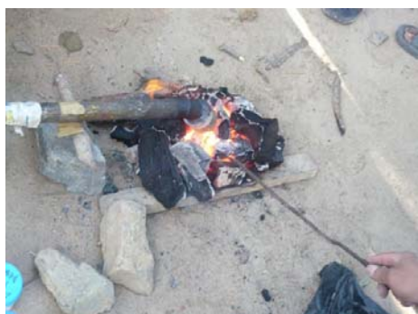
The plastic bag is placed in a ceramic bowl with charcoal and heated. Heating increased with hand powered blower.
