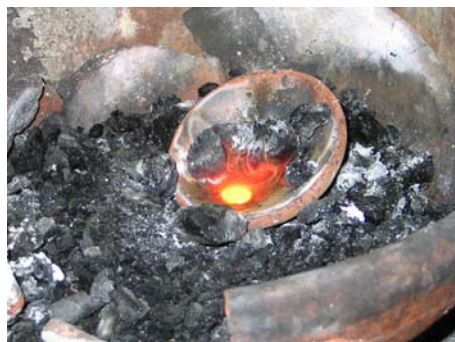
Melting is finished: The shining gold pellet in red glowing molten borax.
