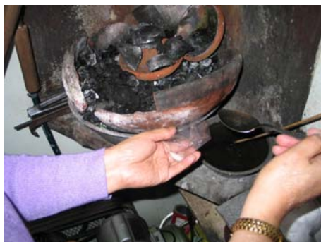
Mineral concentrate in a plastic bag is mixed with borax and a few drops of water.
