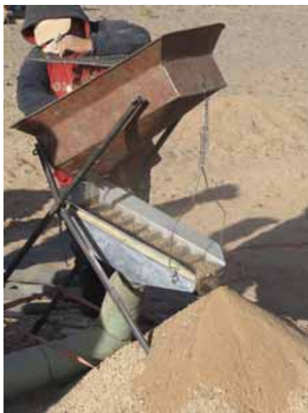
Figure 4. "Dry washing" of gold in the Gobi Desert. The gold is concentrated by means of airflow from an airpump
