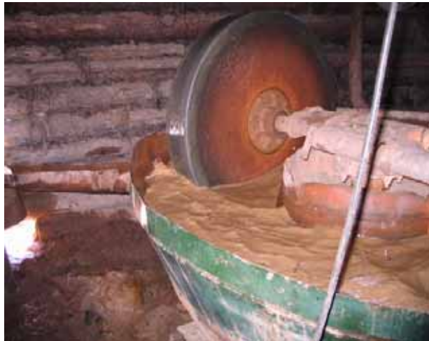
Figure 2. Milling of hard rock gold ore. Five kg of mercury is added for every three to four tons of ore. One third of the mercury is lost directly to the environment with the overflow.
