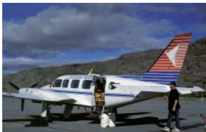
Aircraft (Piper Navajo Chieftain) outfitted for hyperspectral surveying. Kangerlussuaq Airport, 2002.
