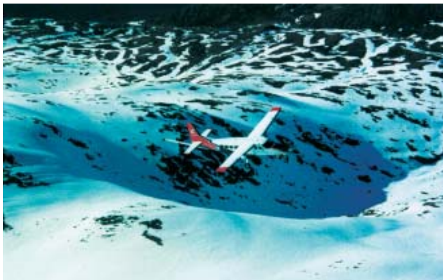
Cessna Grand Caravan from Sander Geophysics Ltd. with tail mounted magnetometer traverses snow-covered terrain at the Nuussuaq peninsula in central West Greenland, Aeromag 1997.
