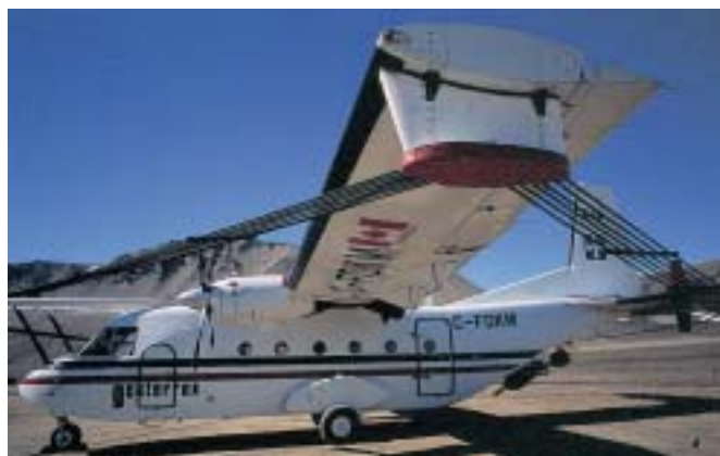
Aircraft (Casa) outfitted for geophysical surveying. The electromagnetic transmitter loop is fixed to the wing tips, tail and nose, Thule Airbase, 1994.
