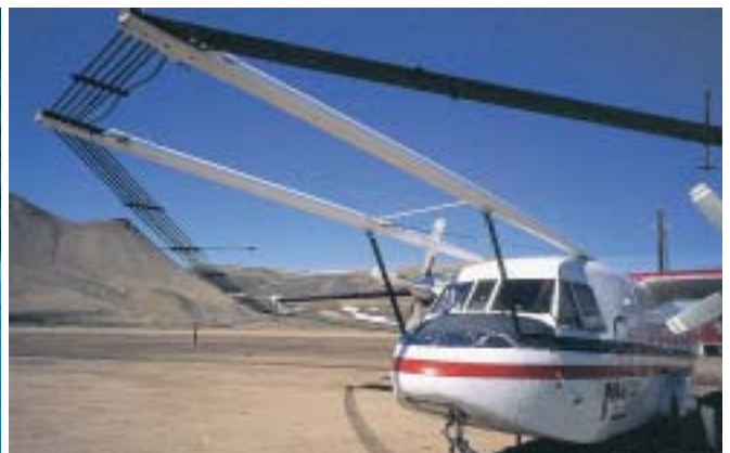
The electromagnetic (GEOTEM) transmitter loop fixed at the nose of the Geoterrex Ltd. Aircraft (Casa), Nuuk, 1995.
