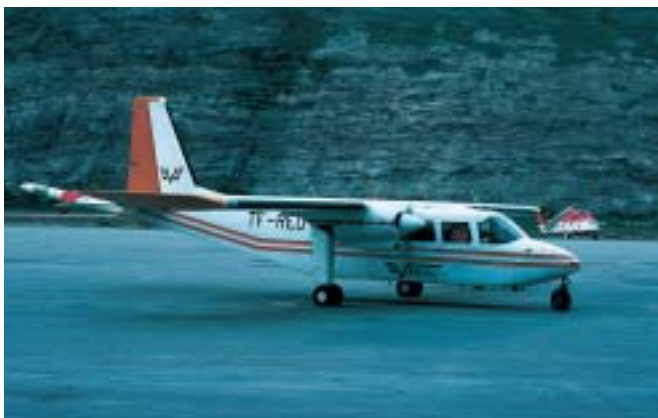
BN-Islander mounted with tail sensor for aeromagnetic surveying. Kangerlussuaq Airport, 1976.
