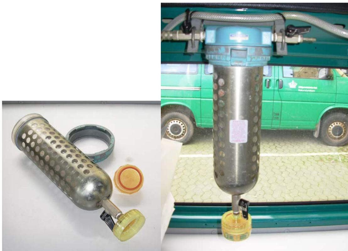
*Figure 3. Pressure filtration equipment from LOOP also used in wells with an insufficient pumping pressure. The figure shows the filter casing and filter holder and field vehicle installation with gas for pressure filtration mounted.*
