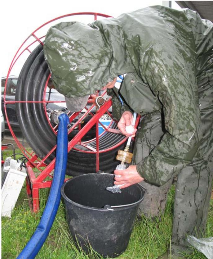
*Figure 2. Online filtration by pumping pressure*
