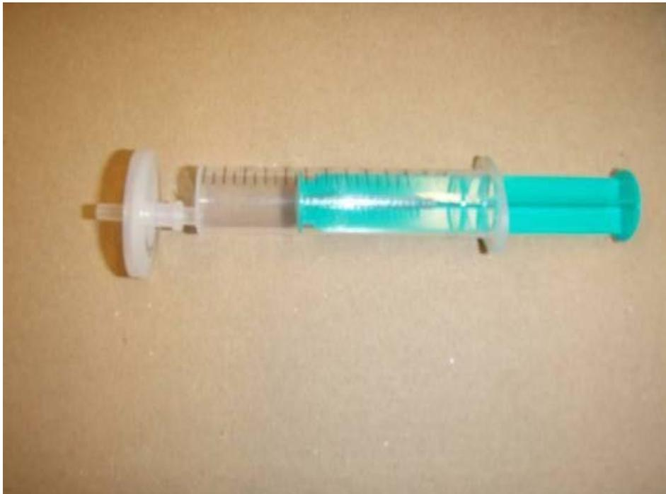
*Figure 4. Hand driven syringe for filtration, with filter unit on the tip.*
